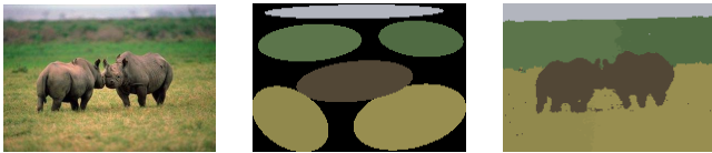
Figure 1. Input image (left). Image modeling via a mixture of Gaussians (center). Image segmentation using the learned model (right).
