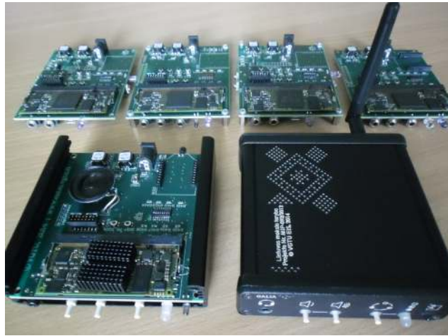
Fig. 3.1. Illustration of six prototypes of speech recognizers (primary versions are on the top, final version is on the bottom)
