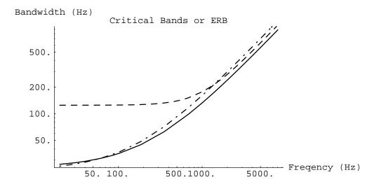
The equivalent filter quality factor, Q, can be determined by dividing center frequency, f, by the ERB. In this plot, the highest curve (sharper filters) corresponds to Glasberg's suggested parameters. The solid curve is the Critical Bank function recommended by Glasberg and Moore, the dashed line is the one by Lyon, and the dash-dot line is from Greenwood
