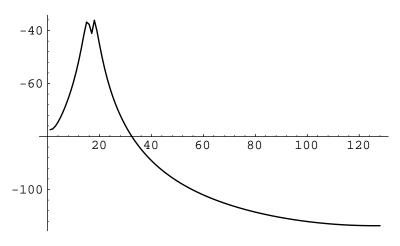
Finally, the all-pole gammatone approximation shown in Section 3.5 has the impulse response shown in the plot below.
