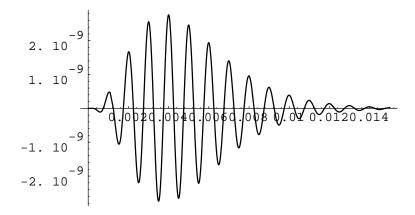
Patterson recommends setting the bandwidth, b, in the Gammatone filter to 1.019 times the ERB.
