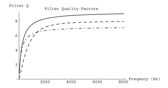
In all three cases the Q is flat, except at low frequencies where the auditory filters have a smaller Q and a wider relative bandwidth. For the rest of this report we will use Glasberg's parameters.
