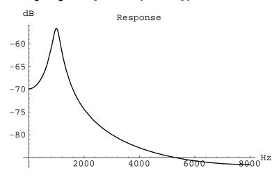
Finally, we can use the **FindImpulseResponse** function to digitally simulate the resulting filter and show its response.
