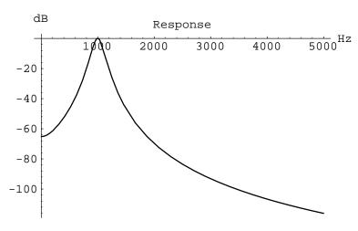
Just to make sure, let's find the 3dB points of this filter. The **FilterSearch** routine finds the frequency that gives an arbitrary response. First, look for the point that is 3dB down in the octave (500->1000 Hz) below the CF, and then find it in the octave above. After determining the 3dB points, the filter's quality factor can be calculated.
