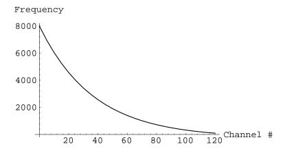
Alternatively, we might know how many channels we want within a frequency range. We can solve the *index* equation for the proper *stepfactor* to use.
