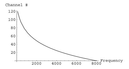
We need to invert this equation to find the mapping between index and center frequency. This will allow us to calculate the appropriate center frequency for any stage in the filter bank.
