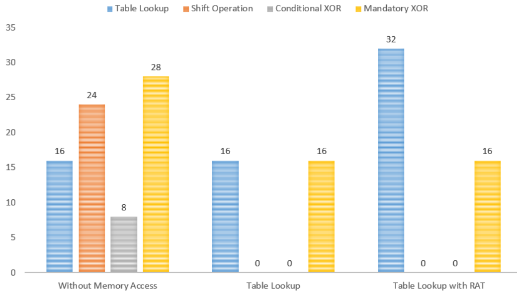
Fig.10. Comparison of RAT with Straightforward AES Implementations in a Single Round. An Implementation that Completely Avoids Memory Access Requires 16 table Lookups, 24 Shift Operations and 36 XOR Operations (8 of which them are Conditional), Whereas Introduction of RAT Incurs 2 times more table Lookups and 16 XOR Operations in a Single Round.
