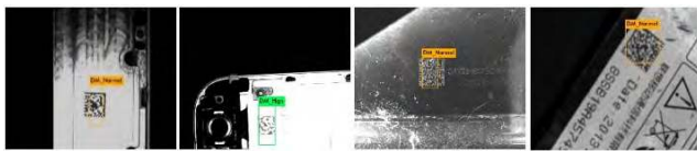
FIGURE 4. Example of inaccurate DPM code location.
