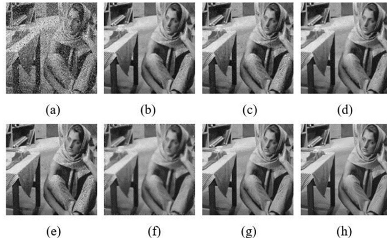
Fig 7. Results of different algorithm in denoised “Barbara” with \sigma = 20 & p_0 = 0.2 : (a) Mixed noise image; (b) NLMNF; (c) CBNLMF; (d) 2013 Zhou’s; (e) 2016 Zhou’s; (f) 2017 Yam’s; (g) Proposed; (h) Original image.
