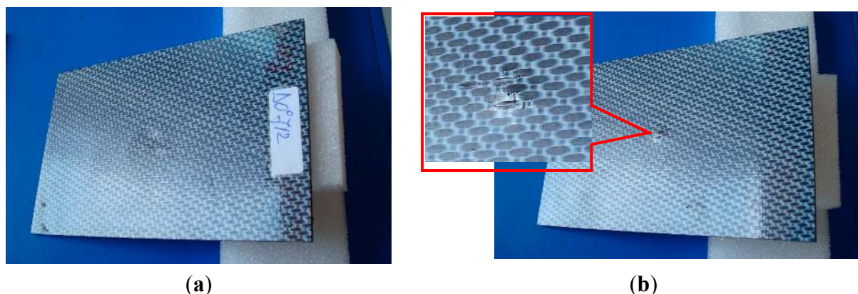
Figure 7. Sample impacted with 12 J energy: (a) front side; (b) back side—inset: breaking of fibers.
