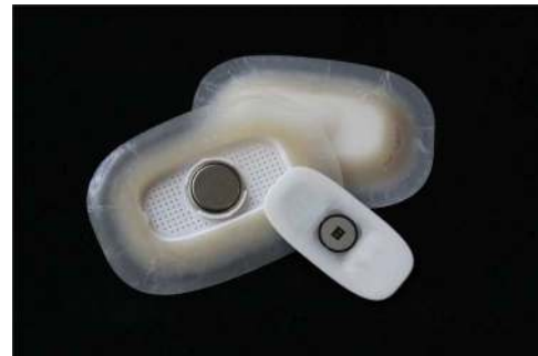
Fig. 1. The picture shows the Electronic Patch with the developed photoplethysmographic sensor. The sensor consist of commercial light emitting diodes and a specially designed annular photodiode. Besides the photoplethysmographic sensor the Electronic Patch also contains electronics for signal processing, wireless radio communication and a coin cell battery. These components are embedded in an hydrocolloid adhesive material. The patch has a size of 88 mm by 60 mm and is 5 mm thick.
