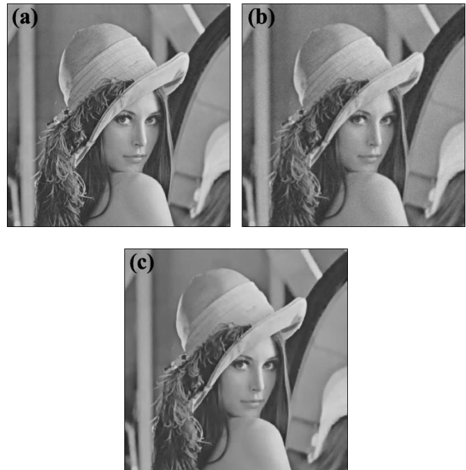
Fig. 6. (a) Original image, (b) blurred image, and (c) restored image using rule (22) and the UDWT-based method.
