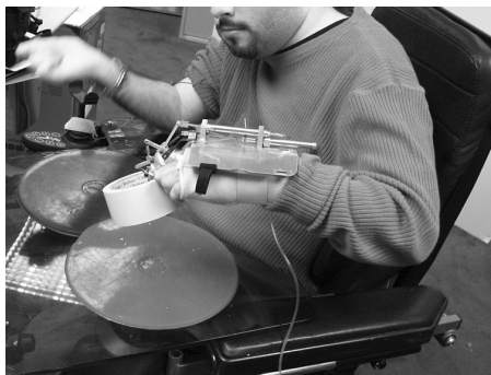
Fig. 3. A spinal cord injured (C5/C6) individual using our orthotic exoskeleton to lift a roll of tape. He has no voluntary control over his hands.
