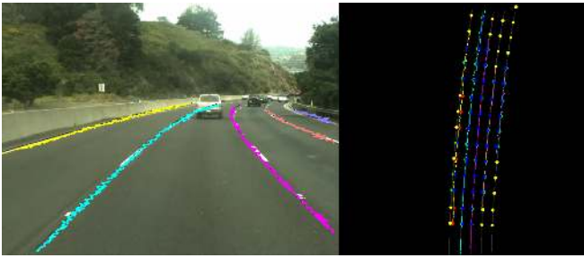
Fig. 7: Left: lane prediction on test image. Right: Lane detection evaluated in 3D
