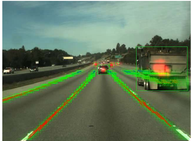
Fig. 1: Sample output from our neural network capable of lane and vehicle detection.
