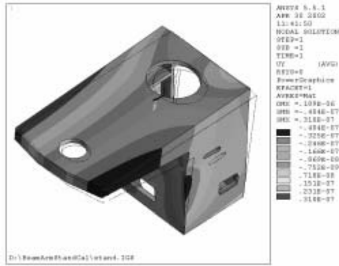
Fig. 19. Bond head stand displacement with 1 N exciting force at point A with small hammer.
