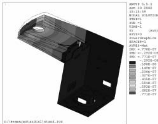
Fig. 20. Bond head stand displacement with 1 N exciting force at point C with big hammer.
