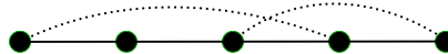
Figure 4: An example of a heavy path graph. The solid path edges are the low-stretch spanning tree of the graph.
