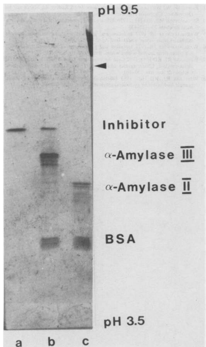
FIG. 3. Protein stain after isoelectric focusing demonstrating the effect of inhibitor on \alpha -amylase II. a, 6 \mu g inhibitor. b, 8 \mu g inhibitor, 10 \mu g \alpha -amylase II, and 10 \mu g BSA. c, 10 \mu g \alpha -amylase II and 10 \mu g BSA.
