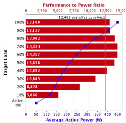
(b) SPECpower_ssj@ 2008 results for a 56-core server hardware from a well-known vendor.
