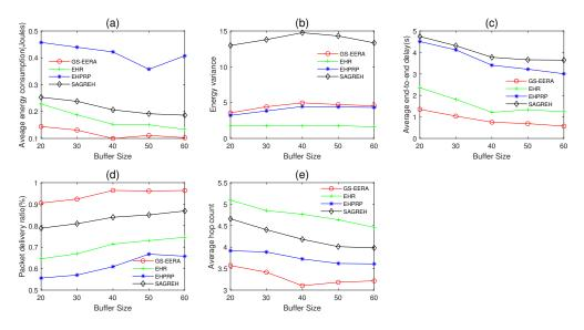
**Figure 13.** The impact of data buffer capacity on (**a**) average energy consumption, (**b**) energy variance, (**c**) average end-to-end delay, (**d**) packet delivery ratio and (**e**) average hop count.
