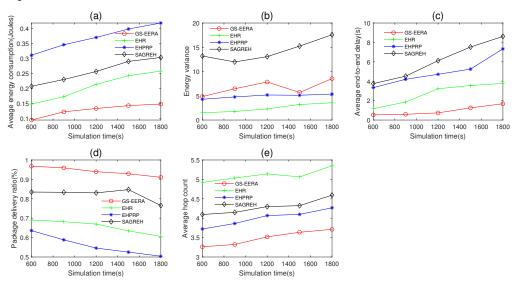
**Figure 12.** The impact of simulation time on (**a**) average energy consumption, (**b**) energy variance, (**c**) average end-to-end delay, (**d**) packet delivery ratio and (**e**) average hop count.
