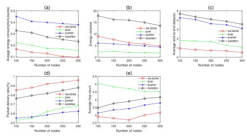
**Figure 10.** The impact of the number of nodes on (**a**) average energy consumption, (**b**) energy variance, (**c**) average end-to-end delay, (**d**) packet delivery ratio and (**e**) average hop count.
