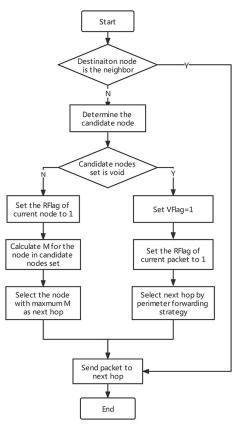
Figure 9. The procedure of GS-EERA main algorithm.
