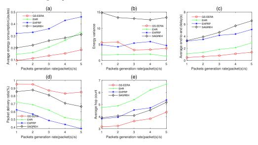
**Figure 14.** The impact of packets generation rate on (**a**) average energy consumption, (**b**) energy variance, (**c**) average end-to-end delay, (**d**) packet delivery ratio and (**e**) average hop count.
