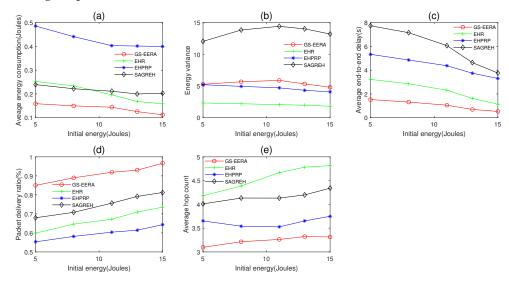
**Figure 11.** The impact of initial energy on (**a**) average energy consumption, (**b**) energy variance, (**c**) average end-to-end delay, (**d**) packet delivery ratio and (**e**) average hop count.
