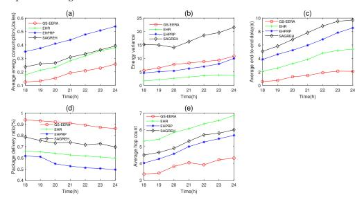
**Figure 15.** The performance change with time. (**a**) average energy consumption, (**b**) energy variance, (**c**) average end-to-end delay, (**d**) packet delivery ratio and (**e**) average hop count.
