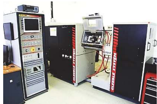
FIGURE 5: The Gleeble 3800 thermomechanical simulator [6].
