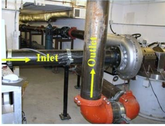
Fig. 1. Photograph of the experimental setup, including the direction of the inlet and the outlet air flow.
