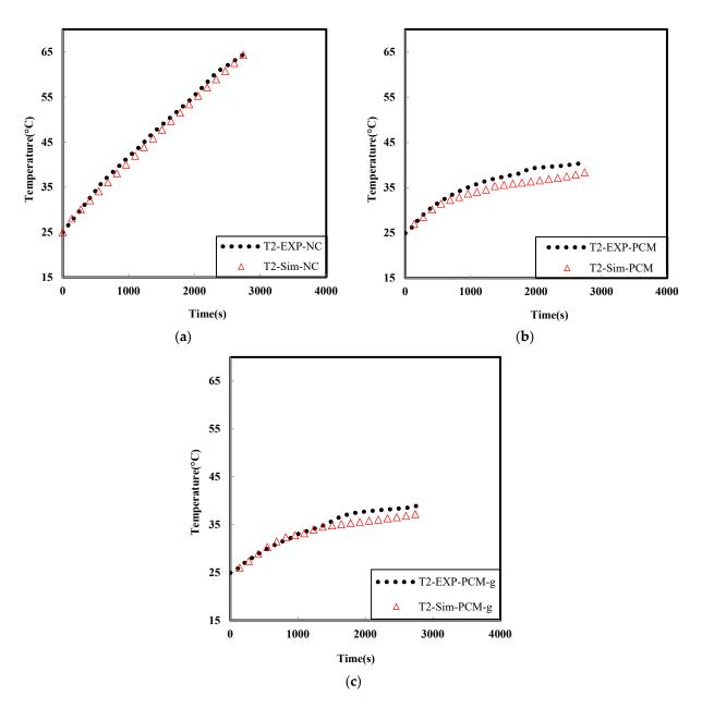
**Figure 7.** Thermal model validation of the module (a) under natural convection, (b) PCM, and (c) PCM-graphite at a 1.5C discharging rate (Sim: Simulation, NC: Natural convection, PCM-g: PCM-graphite.
