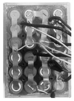
**Figure 5.** The temperature curve of the battery module and an image of the test setup using PCM under a 1.5C discharging rate.
