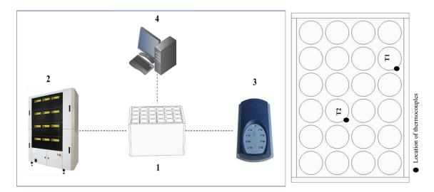
**Figure 2.** (**left**) The picture of the test setup comprising (1) the battery module, (2) battery tester, (3) data logger, (4) personal computer, (**right**) and the location of the thermocouples.
