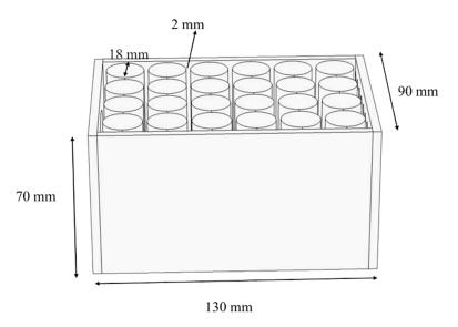
**Figure 1.** Schematic of the battery module with dimensions.
