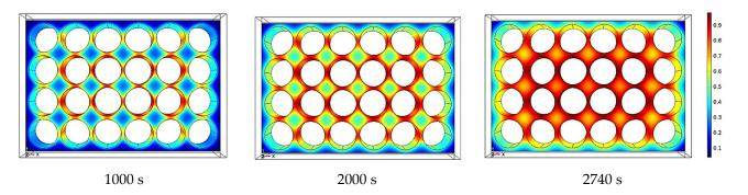
**Figure 10.** Liquid fraction contour of the PCM-graphite after 1000, 2000, and 2740 s under a 1.5C discharging rate.
