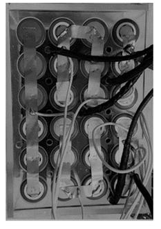
**Figure 3.** The temperature curve of the battery module and an image of the test setup for natural convection under a 1.5C discharging rate (EXP: Experimental).
