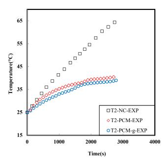
**Figure 6.** The comparison of the  $T_2$  thermocouple under the different cooling technologies (NC: natural convection, PCM-g: PCM-graphite).
