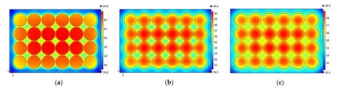
**Figure 8.** Temperature contour of the module using (a) natural convection (NC), (b) PCM, and (c) PCM-graphite (PCM-g) cooling methods under a 1.5C discharging rate.
