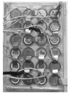
**Figure 4.** The temperature curve for the battery module and an image of the test setup using PCM under a 1.5C discharging rate.
