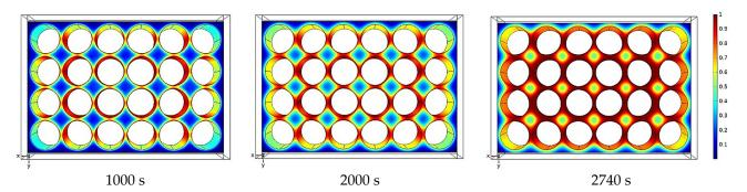
**Figure 9.** Liquid fraction contour of the PCM after 1000, 2000, and 2740 s under a 1.5C discharging rate.
