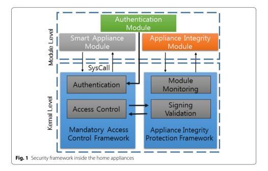
not influence a running module and monitors an attack action. This framework is made up of smart appliance module, appliance integrity module, mandatory access control framework, and appliance integrity protection framework.
