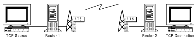
Figure 4. Simulation setup. TCP source and destination are connected over two routers that have a wireless link in between.
