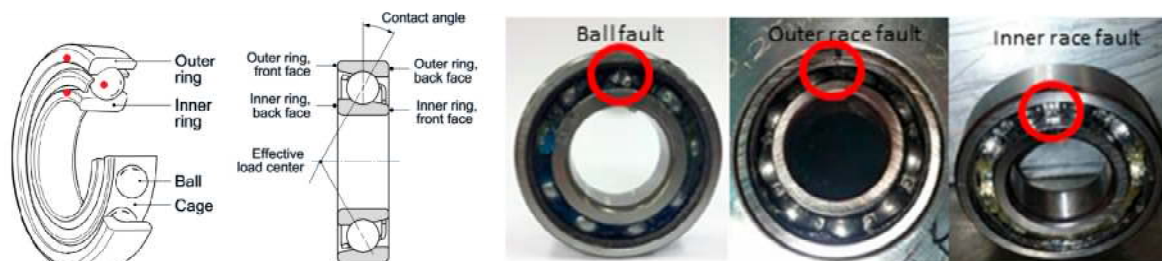
Figure 4. Bearing Structures and Fault Location Sketch Map.
