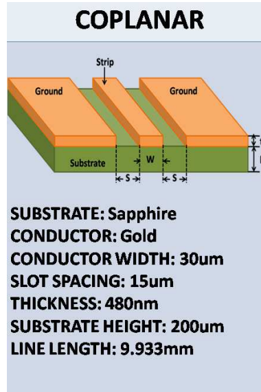
Figure 6: Geometry of the Gold Coplanar Waveguide used as the Benchmark
