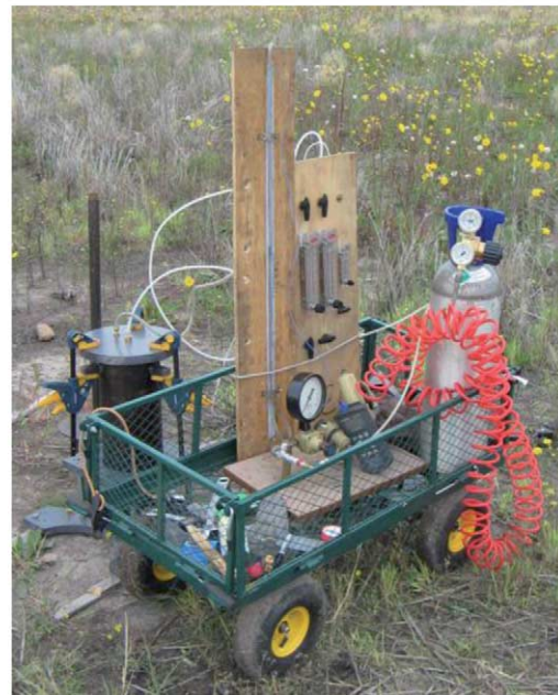
Fig. 1. The schematic and prototype of portable air permeameter.
