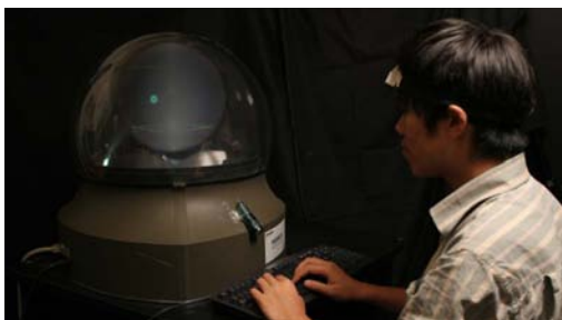
Figure 3. Volumetric display setup. The electromagnetic tracker measures head movement to allow for imagery to be displayed only when head position is within a given range.
