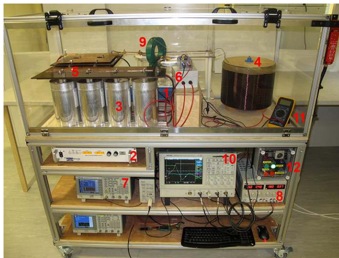
Fig. 2. HV Test Rig Components: 1- Thermal Conditioner 2- 12 kV Power Supply 3- 6.5 kV Bank Capacitors 4- 75mH Inductor 5- Copper Plates 6- Gate Driver 7- Signal Generator 8-Current Supply 9-Current Probe 10- Oscilloscope 11-Voltmeter 12- Interlock
