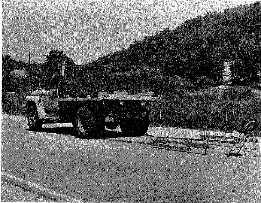
Figure 1: Benkelman Beam Deflection Test Setup
