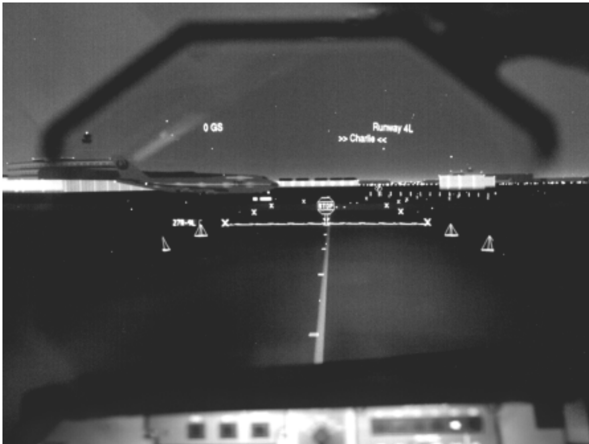
Figure 1. Photograph showing the T-NASA HUD symbology overlaid on the out-the-window night view approaching Runway 27R/9L on Taxiway Charlie at Chicago O'Hare. The cleared taxiway is demarcated by the series of rectangular centerline markers and the side cones. Hold short symbology includes the virtual stop sign, virtual stop bar, and the replacement of the side cones with "X"s at and past the stop bar. Note the A/C taking off on 27R/9L (upper left of figure).
