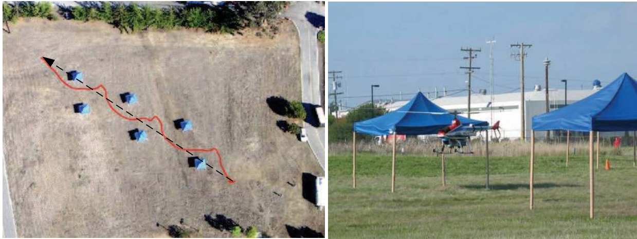
Figure 12. Aerial view of urban navigation experiment (dashed: given straight path, solid: actual flight path of UAV during experiment)
