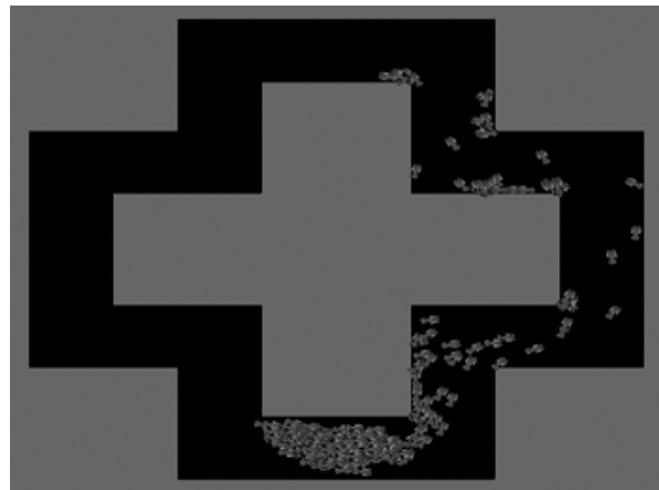
Fig. 1. The training course is shown during a training run. The population has converged such that there are many similar individuals, as can be seen by the large number of cars in a similar position on the track.
