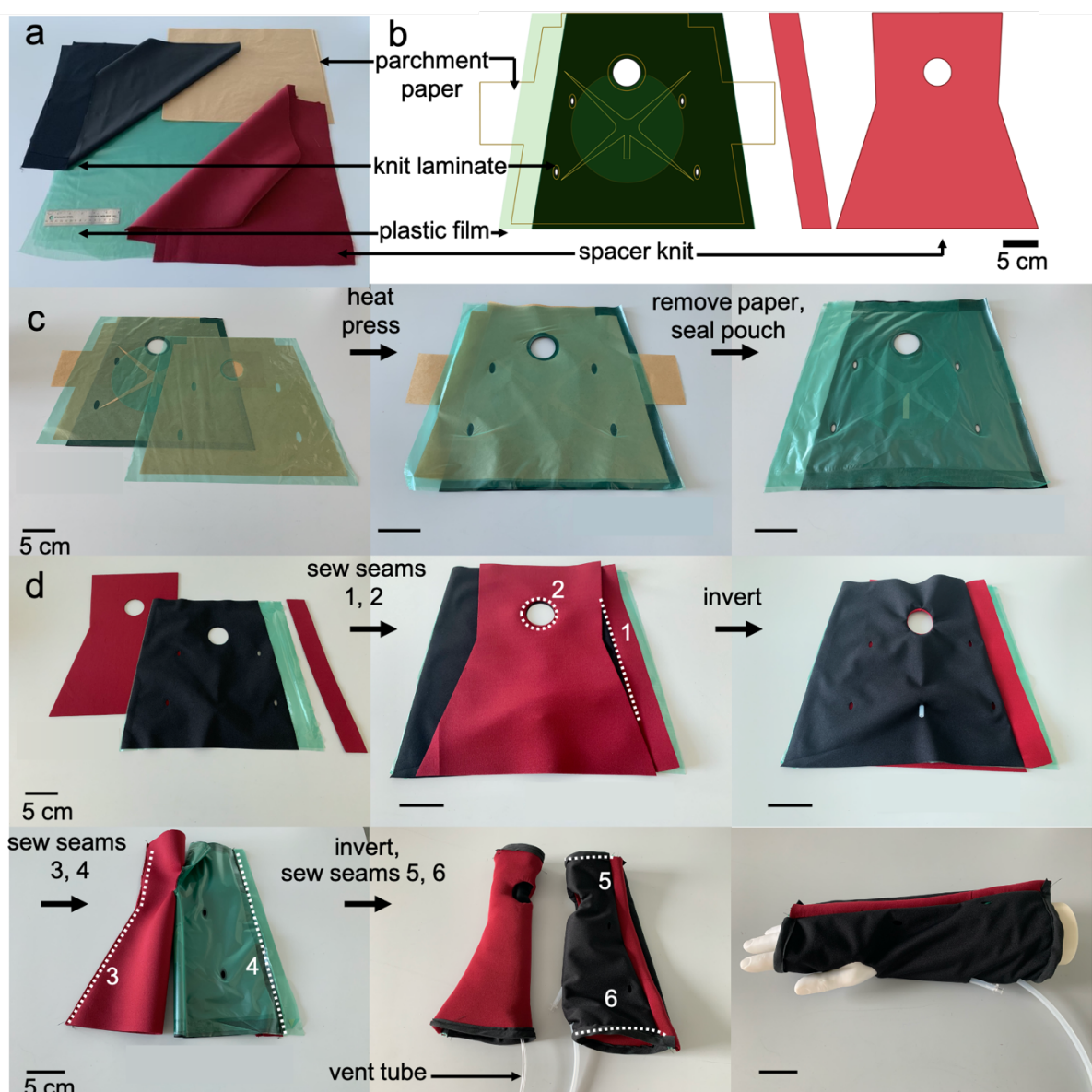
Figure 2. Fabrication process. (a) Photograph of sheets of materials used in fabrication of the FFC. (b) Schematic diagram of the pattern used to laser cut these materials. (c) Photographs of the cast at various stages of the fabrication process. Heat pressing, with patterns of parchment paper as sacrificial layers, is used to fabricate the thermoplastic pouch and fluidic channels for the foam. The red fabric pieces are sewn to the black fabric containing the green pouch (seams 1 and 2). The red fabric is then inverted through the thumbhole and seams 3 and 4 are sewn. Finally, the garment is inverted again, and the top and bottom seams (5 and 6) complete the fabrication process. A more detailed figure describing the fabrication process can be found in the Supporting Information, Figure S1 .
