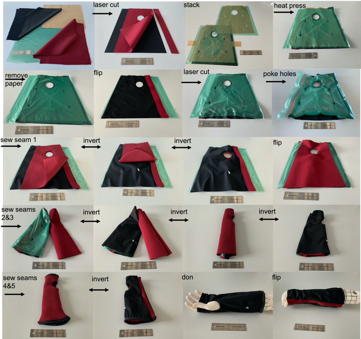
Figure S1. Fabrication process, extended version. Photographs of each step of the fabrication process, including laser cutting, heat pressing, and sewing of the cast.
