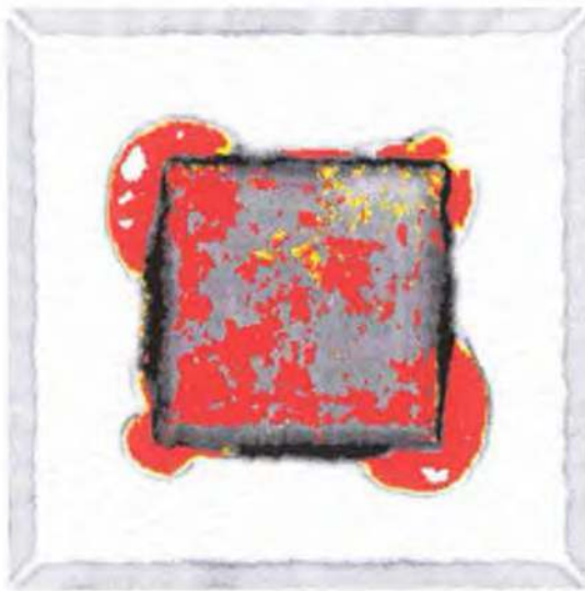
(i) Package design I, die-paddle interface
