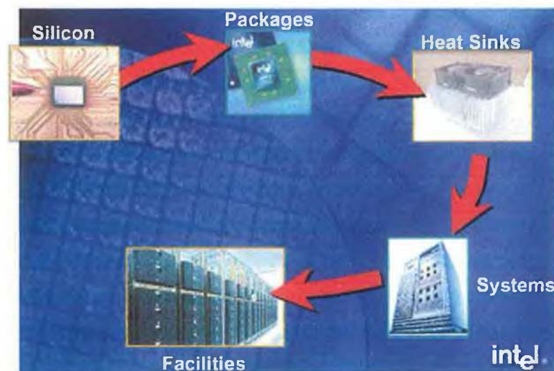
Figure 1.3 Thermal analysis chain of an electronic system, from IC to data centre [21].
