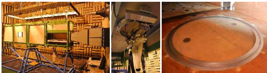
Fig. 6 From the left to the right, whole view of the channel flow, rear view of the rotating disk and view of the pressure antenna on the front side of this disk.
