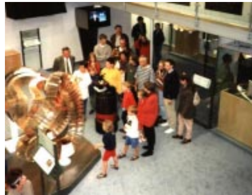
Fig. 10. Typical situation in which several people surrounded the robot and lead to measurement errors.
