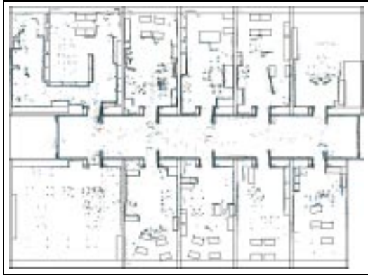
Fig. 2. Overlay of a hand-crafted CAD map of the office environment used for the experiments and the corresponding map learned by scan matching.
