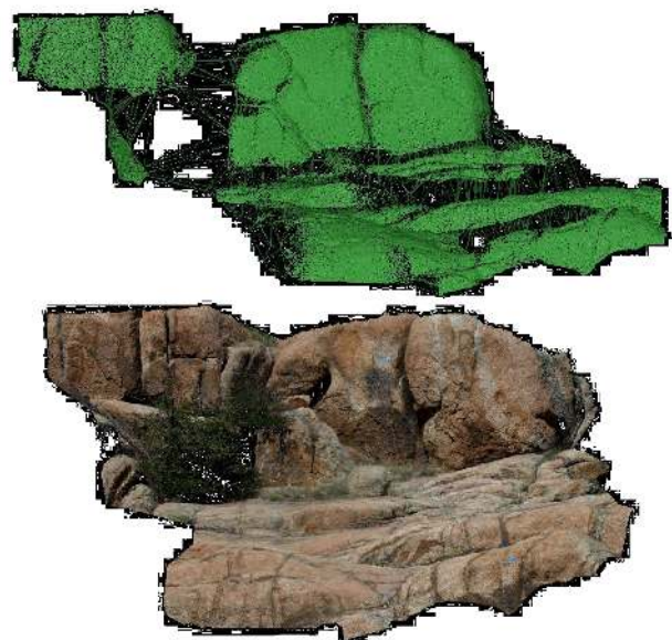
Figure 11: Model produced at Granite Dells (15 x 10 m) - (top) wireframe model - (bottom) same model with draped images
