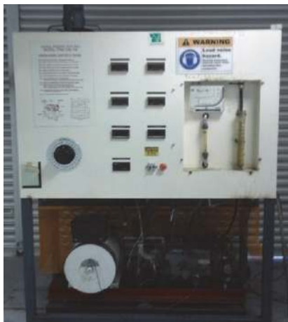
FIGURE 3: Diesel Engine Performance Test Bed (Techno-mate, TNM-TDE-700).
