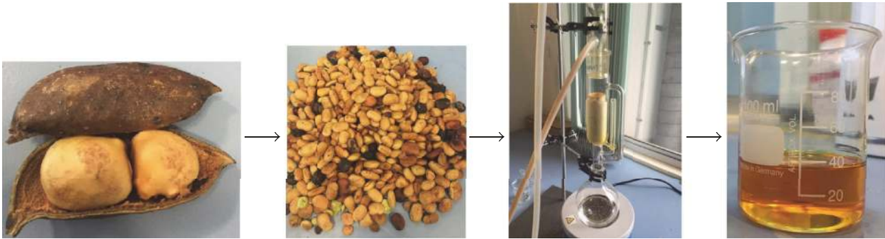
FIGURE 1: Crude karanja oil extraction process.
