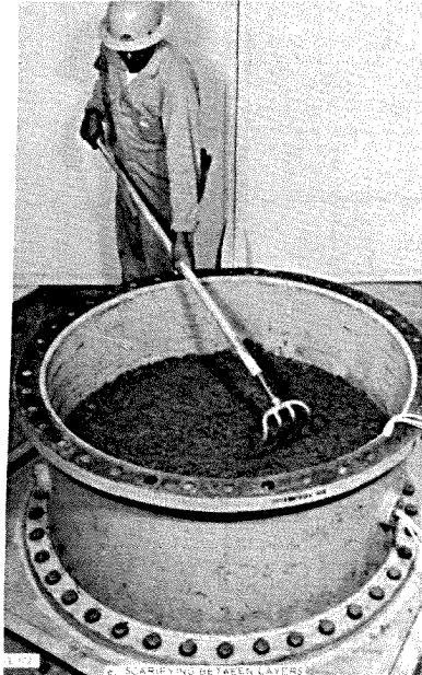
e. SCARIFYING BETWEEN LAYERS
