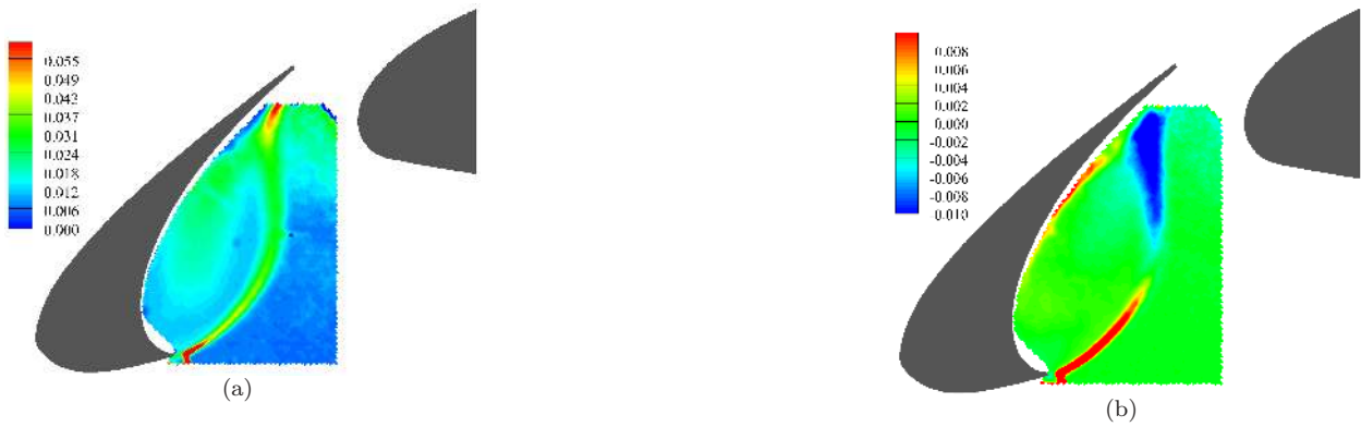
Figure 16. Turbulence quantities, (a) TKE, 1/2(\langle u'u' \rangle + \langle v'v' \rangle + \langle w'w' \rangle) / U_\infty^2 and (b) Reynolds stress component \langle u'v' \rangle / U_\infty^2 .
