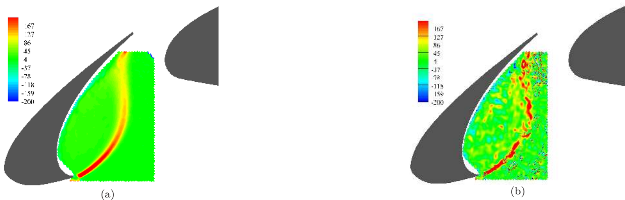
Figure 14. Spanwise vorticity, \omega_z c / U_\infty , (a) averaged and (b) instantaneous.
