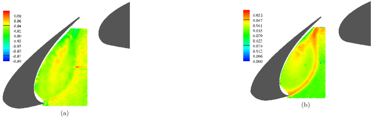
Figure 15. Spanwise velocity component (a) mean, \langle w \rangle / U_\infty and (b) rms, \langle w' \rangle / U_\infty .
