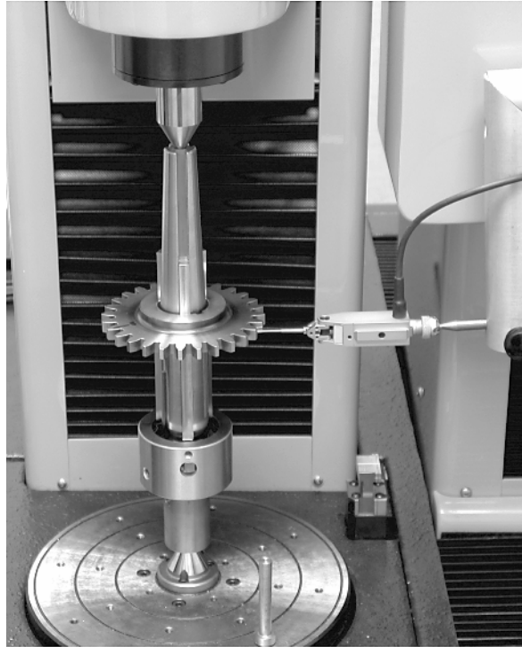
Figure 4.—A test gear while being inspected on the gear coordinate measurement machine.
