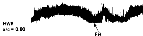
Figure 7.- Response of hot-wire anemometer probe installed near trailing edge of the Vertol VR-7 airfoil during oscillation in pitch.
