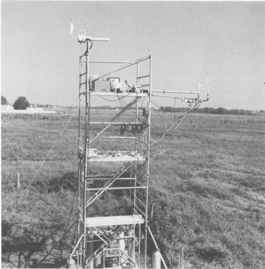
Fig. 3. A photograph of the 7 m scaffolding tower from which eddy correlation and other meteorological measurements were made. Note the horizontal boom carrying velocity sensors for covariance measurements, the long sampling inlet tube for drawing air samples into the particulate and gaseous sulfur analyzers, and the flexible sampling hoses for the other air chemistry sensors. Equipment was arranged on the tower to minimize the obstruction to wind flow.
