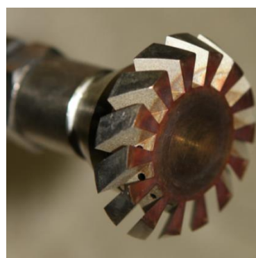
Fig. 2.2d Cross-sectional view of fuel nozzle. Fig. 2.2e Direct photo of tested fuel nozzle.
