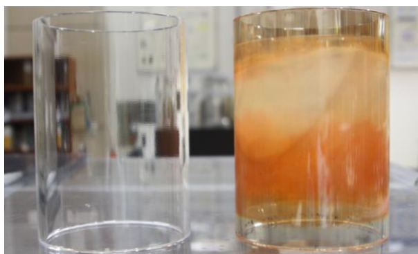
Fig. E.1 Comparison of quartz tubes between before (left) and after (right) burning of CO containing fuels.
