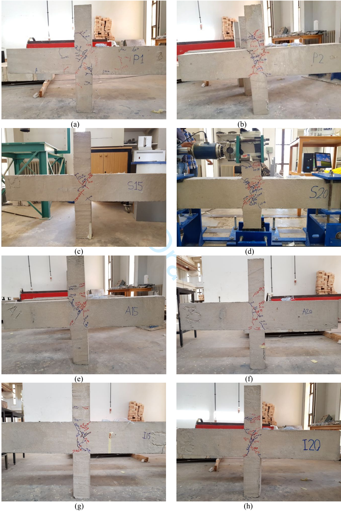
Figure 1 The level of damage and crack patterns of all test specimens
