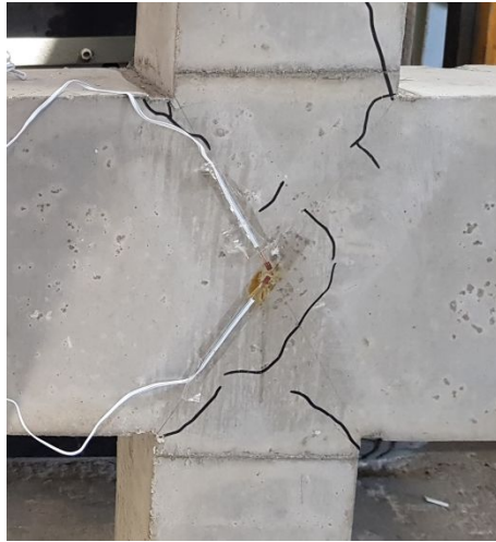
Figure 1 Strain gauges location
