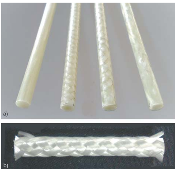
Figure 3. (a) Some manufactured rods and (b) a specimen after burn-off test
