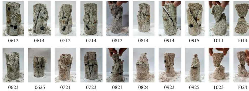
FIGURE 3: Failure patterns of the specimens.
