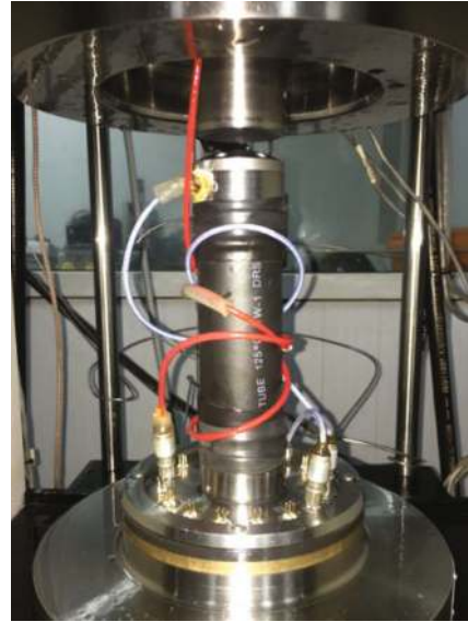
FIGURE 3: Permeability experimental device.
