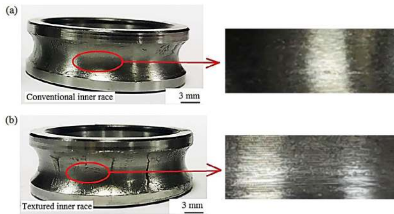
Fig. 11 Photographic view of inner races after the experiment (load = 60 N, speed = 1,400 rpm (3.4 m/s), DAD = 15%). (a) Visual of inner race (conventional bearing) and (b) visual of textured inner race (textured bearing).
