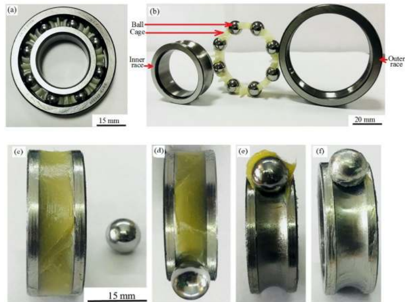
Fig. 1 Photographic views of a radial deep groove ball bearing and pushing aside of grease employed in lubrication. (a) Assembled ball bearing; (b) components of ball bearing; (c) grease filled track on inner raceway; (d) one ball positioned on track at inner raceway; (e) removal of grease from raceway when a ball moves; (f) track view of inner raceway after few passes of a ball.
