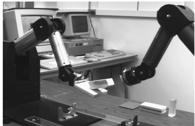
Figure 1: The experimental setup consists of two Zebra robots, with flat palms attached to each wrist. The Zebras are shown manipulating an irregular block.
