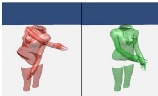
Fig. 8. Demonstration of magnetic compensation technique—(left—feedback when using magnetometer data in a magnetically polluted environment, Torso, and upper-arm are severely affected by magnetic interference during real-time use; right—feedback using context specific magnetometer data from previous recordings during real-time use, Torso, and upper-arm provide contextually relevant data and respond as if magnetic interference was not present).
