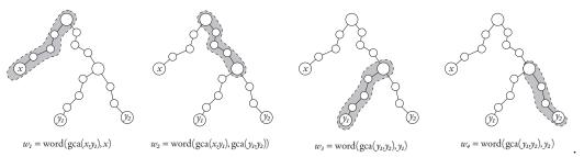
A regular query  $\varphi[x, y_1, y_2]$  is called *path-based* if its truth value depends only on some regular properties of the four words  $w_1, \ldots, w_4$ . The precise definition of path-based queries we use in this paper is in terms of monoids. A query that selects triples only in arrangement (A1) is called *path-based* if there exists a monoid morphism
